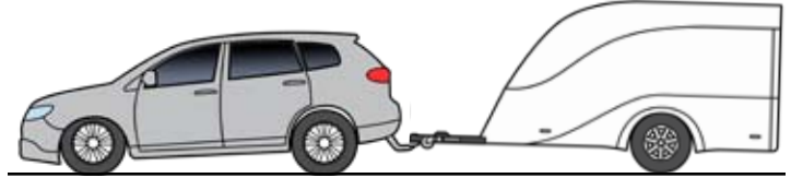
Incorrect weight distribution in trailer
